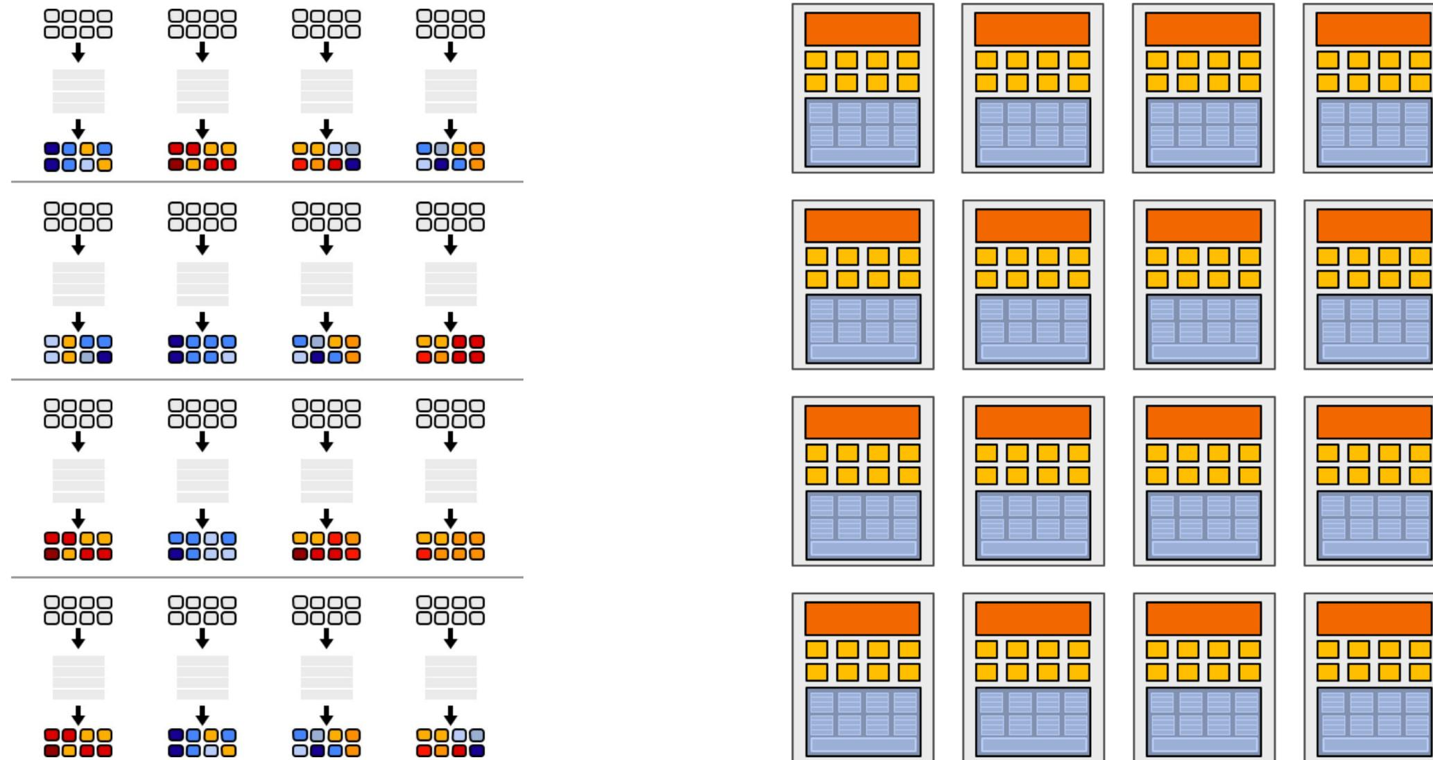
**16 cores x 8 ALUs/core = 128 ALUs 16 cores = 16 simultaneous instruction streams**
